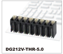
DG212V-THR-5.0 500B/17.5A 0.2-1.5mm 2 300B/12A 28-14AWG Полосов 2P-24P
