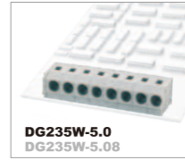
DG235W-5.0 DG235W-5.08 250B/15A 0.2-2.5 SOL 0.2-1.5 STR 300B/5A 20-18AWG Полосов 1P-XXP
