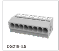
DG219-3.5 320B/17.5A(III/2) 0.2-1.5mm 2 300B/10A 24-16AWG Полосов 2P-XXP
