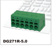
DG271R-5.0 400B/24A(III/2) 0.2-4.0mm 2 300B/20A 24-12AWG Полосов 1P-XXP
