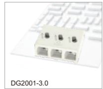
DG2001-3.0 160B/9A 0.14-0.34mm 2 320B/3A 26-22AWG Полосов 1P-3P
