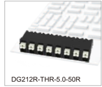
DG212R-THR-5.0-50R 500B/17.5A 0.2-1.5mm 2 300B/12A 28-14AWG Полосов 2P-12P
